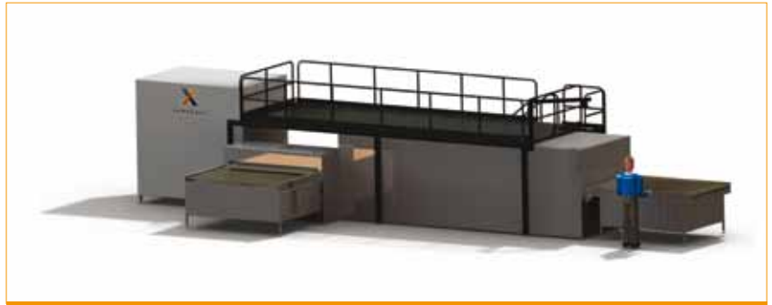
Figure 4. A rendering of Xerocoat's turnkey antireflective coating equipment for PV module production lines.
